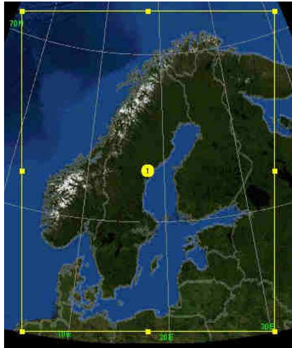
Fig. 2: Domain of the anemos wind atlas Scandinavia / Baltic 10 km. Domain with 10 x 10 km 2 .
